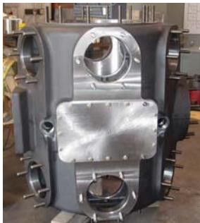
The new ACI custom engineered cylinder required a bottom mounting pad, top inlet and side discharge in order to “bolt-in” to existing foundations and piping.
