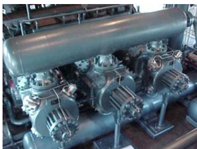
Fig. 3 Completed KVG 3600 with the ACI re-engineered cylinder on center throw.
