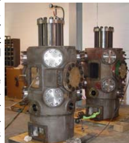
Fig. 2 Cylinder Hydro-testing at ACI Shop.
