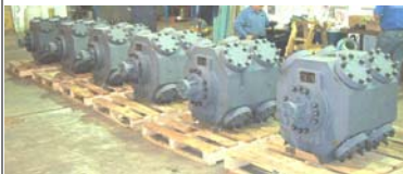
Six (6) 10-in, 1500 psig (103.4 bar) MAWP cylinder assemblies prior to shipment to the compressor station.
