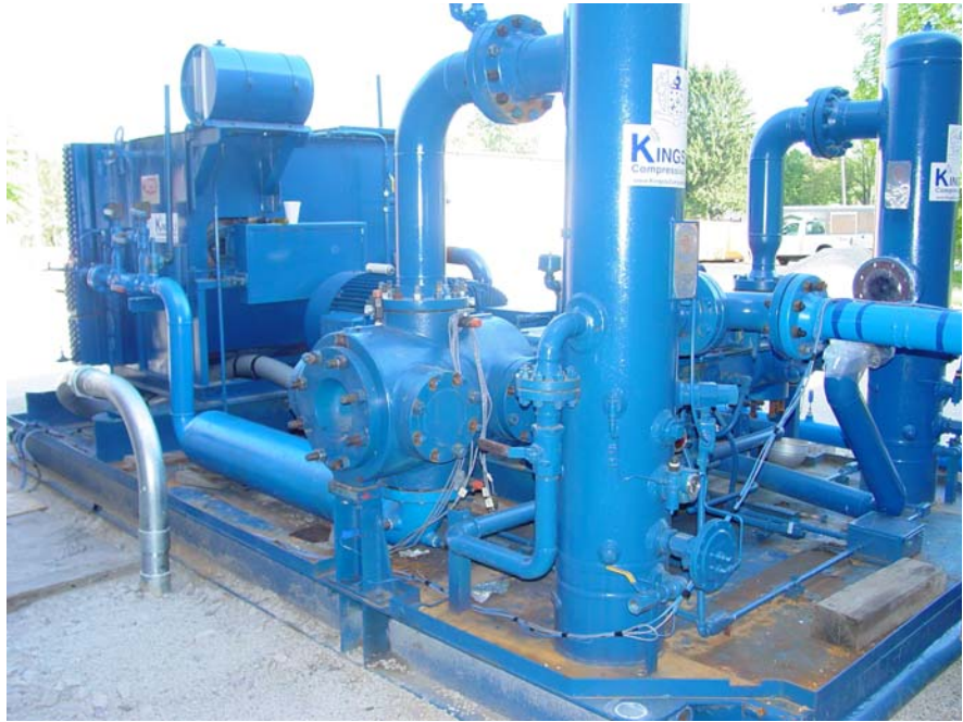
Figure 10: 200 HP, 600 to 1200 RPM Closed Loop Test Facility Dedicated to Valve & Unloader Testing
